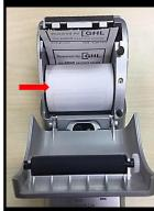
2. Drop in the paper roll with the paper pulling from the back and out the top of the roll.
