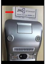
3. It is important the lid is fully closed so that the paper roll fully engages the paper.
